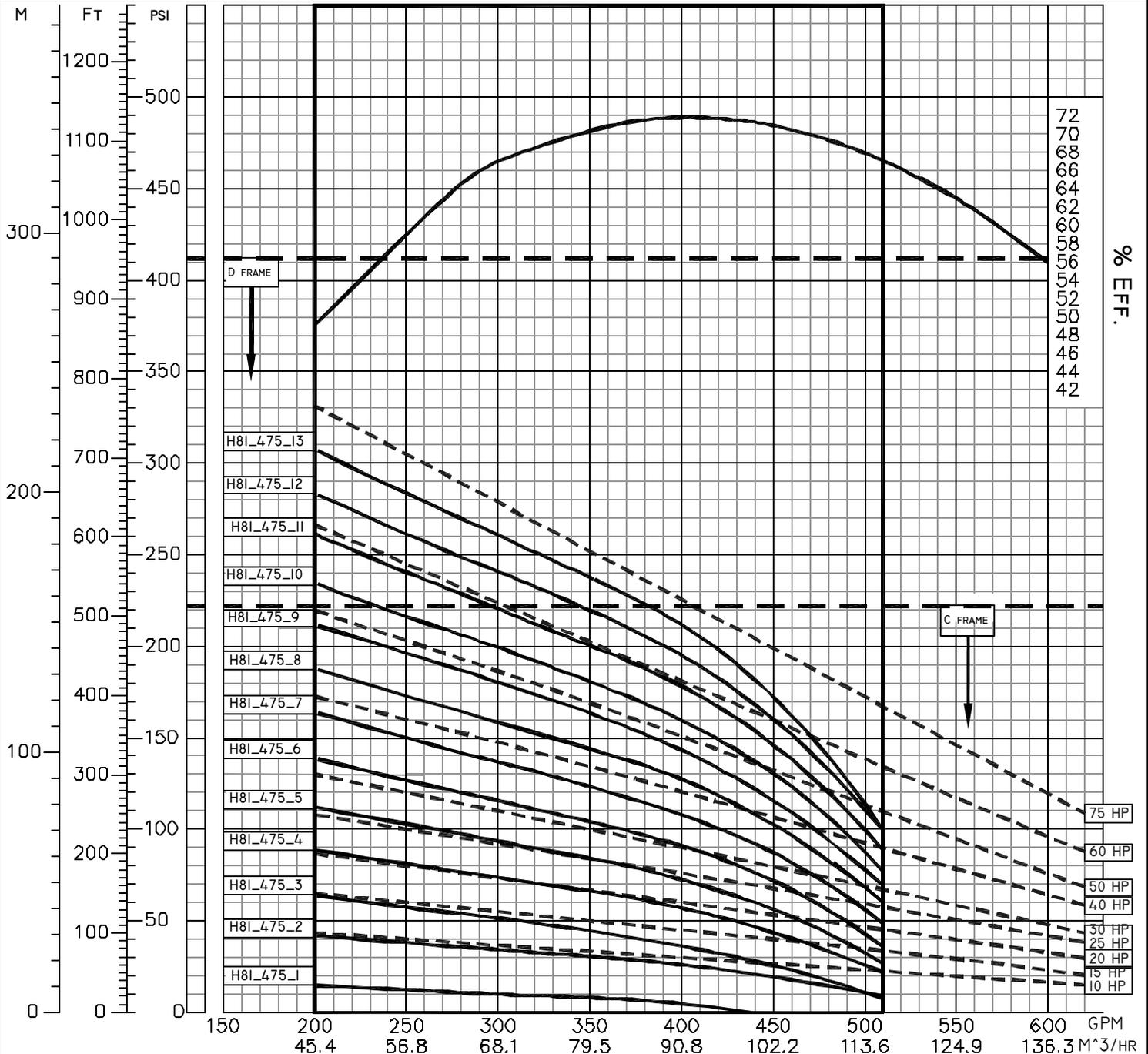
PERFORMANCE IS BASED ON 2900 (NOMINAL) RPM, 50 HZ MOTOR. THESE PUMP CURVES AND ANY INDIVIDUAL CURVES, WHICH ARE AVAILABLE UPON REQUEST, ARE TYPICAL ONLY AND ARE NOT GUARANTEED AS MINIMUM PERFORMANCE. IF EXACT FLOW AND PRESSURE ARE REQUIRED, A CERTIFIED CURVE MAY BE ORDERED AT ADDITIONAL COST IF ACCOMPANIED BY AN ORDER AND ONLY AFTER PUMP HAS BEEN TESTED.
