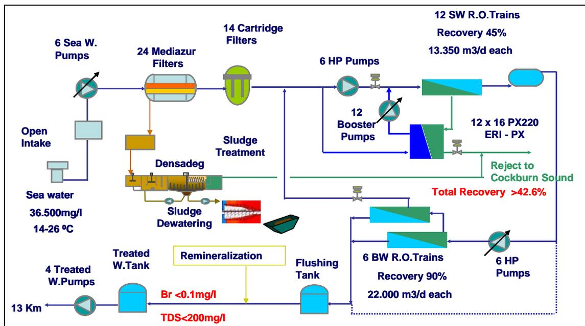
Figure 1 Perth seawater desalination plant process diagram
