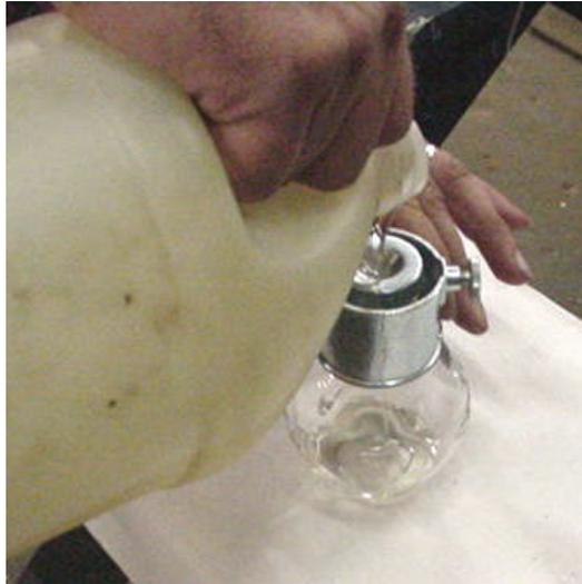
14. To fill the D frame bearing housing with oil, place the reservoir on its top and fill the reservoir to where glass globe joins to the metal base.
