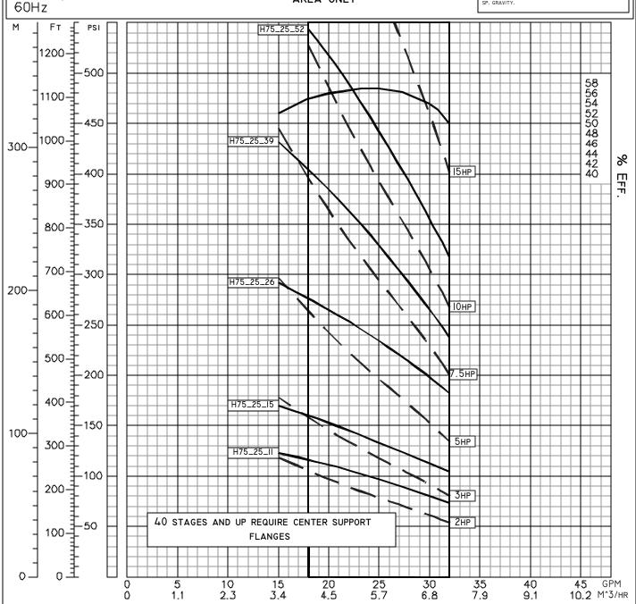
PERFORMANCE IS BASED ON 3600 (NOMINAL) RPM, 60 HZ MOTOR. THESE PUMP CURVES AND ANY INDIVIDUAL CURVES, WHICH ARE AVAILABLE UPON REQUEST, ARE TYPICAL ONLY AND ARE NOT GUARANTEED AS MINIMUM PERFORMANCE. IF EXACT FLOW AND PRESSURE ARE REQUIRED, A CERTIFIED CURVE MAY BE ORDERED AT ADDITIONAL COST IF ACCOMPANIED BY AN ORDER AND ONLY AFTER PUMP HAS BEEN TESTED.
