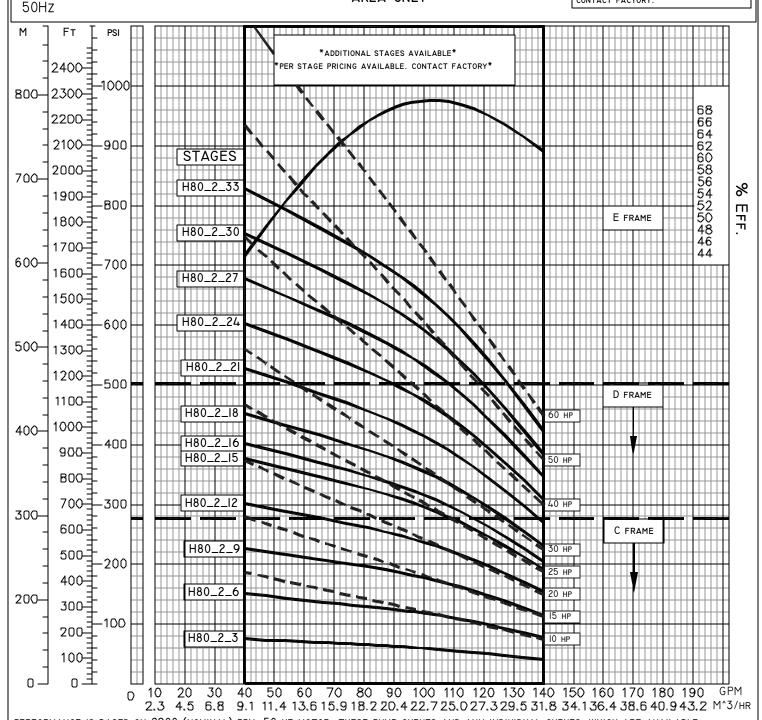
PERFORMANCE IS BASED ON 2900 (NOMINAL) RPM, 50 HZ MOTOR. THESE PUMP CURVES AND ANY INDIVIDUAL CURVES, WHICH ARE AVAILABLE UPON REQUEST, ARE TYPICAL ONLY AND ARE NOT GUARANTEED AS MINIMUM PERFORMANCE. IF EXACT FLOW AND PRESSURE ARE REQUIRED, A CERTIFIED CURVE MAY BE ORDERED AT ADDITIONAL COST IF ACCOMPANIED BY AN ORDER AND ONLY AFTER PUMP HAS BEEN TESTED.
