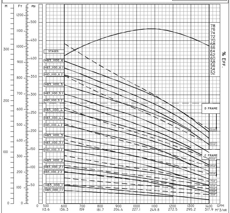
PERFORMANCE IS BASED ON 3600 (NOMINAL) RPM, 60 HZ MOTOR. THESE PUMP CURVES AND ANY INDIVIDUAL CURVES, WHICH ARE AVAILABLE UPON REQUEST, ARE TYPICAL ONLY AND ARE NOT GUARANTEED AS MINIMUM PERFORMANCE. IF EXACT FLOW AND PRESSURE ARE REQUIRED, A CERTIFIED CURVE MAY BE ORDERED AT ADDITIONAL COST IF ACCOMPANIED BY AN ORDER AND ONLY AFTER PUMP HAS BEEN TESTED.
