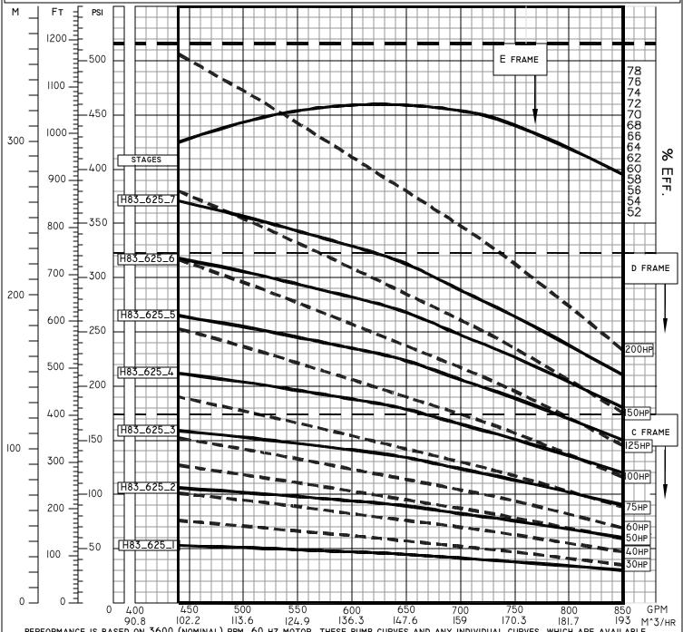
PERFORMANCE IS BASED ON 3600 (NOMINAL) RPM, 60 HZ MOTOR. THESE PUMP CURVES AND ANY INDIVIDUAL CURVES, WHICH ARE AVAILABLE UPON REQUEST, ARE TYPICAL ONLY AND ARE NOT GUARANTEED AS MINIMUM PERFORMANCE.  $\pm$  6% PSI and  $\pm$  8% GPM. IF EXACT FLOW AND PRESSURE ARE REQUIRED, A CERTIFIED CURVE MAY BE ORDERED AT ADDITIONAL COST IF ACCOMPANIED BY AN ORDER AND ONLY AFTER PUMP HAS BEEN TESTED.
