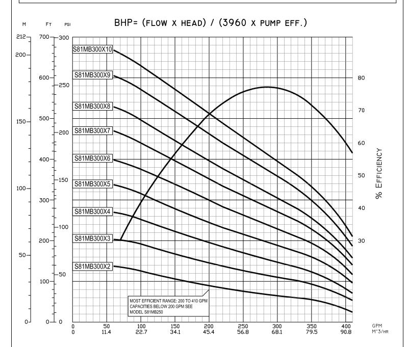
PERFORMANCE IS BASED ON 3600 (NOMINAL) RPM, 60 HZ MOTOR. THESE PUMP CURVES AND ANY INDIVIDUAL CURVES, WHICH ARE AVAILABLE UPON REQUEST, ARE TYPICAL ONLY AND ARE NOT GUARANTEED AS MINIMUM PERFORMANCE. IF EXACT FLOW AND PRESSURE ARE REQUIRED, A CERTIFIED CURVE MAY BE ORDERED AT ADDITIONAL COST IF ACCOMPANIED BY AN ORDER AND ONLY AFTER PUMP HAS BEEN TESTED.
