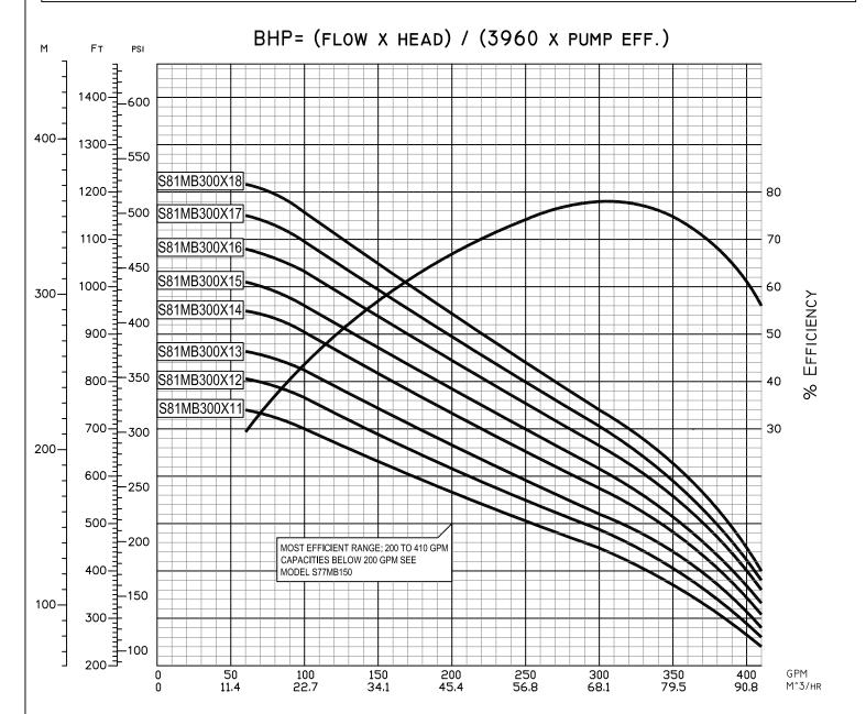
PERFORMANCE IS BASED ON 3600 (NOMINAL) RPM, 60 HZ MOTOR. THESE PUMP CURVES AND ANY INDIVIDUAL CURVES, WHICH ARE AVAILABLE UPON REQUEST, ARE TYPICAL ONLY AND ARE NOT GUARANTEED AS MINIMUM PERFORMANCE. IF EXACT FLOW AND PRESSURE ARE REQUIRED, A CERTIFIED CURVE MAY BE ORDERED AT ADDITIONAL COST IF ACCOMPANIED BY AN ORDER AND ONLY AFTER PUMP HAS BEEN TESTED.
