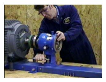
The bearing frame can now be removed from the bedplate.
