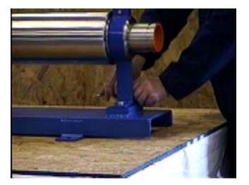
Remove the casing bolts that secure the pump casing assembly to the casing adapter assembly.
