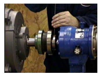
Slide the coupling on the motor shaft back towards the motor.
