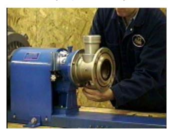
Pull the casing adapter assembly away from the bearing frame in a horizontal direction. Be careful not to damage the mechanical seal housing o-ring or misplace it.
