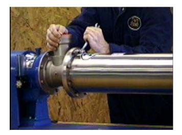
Separate the pump casing assembly from the casing adapter assembly. Do not pull the casing off of the pump staging. The pump casing assembly and the pump staging must be removed together. The pump shaft has a hex end, which plugs into the shaft coupler. There are no threads so the shaft will simply pull out of the shaft coupler. Be careful not to damage the o-ring that seals the pump casing and the casing adapter. Do not discard the o-ring. Use two people to remove the casing assembly.
