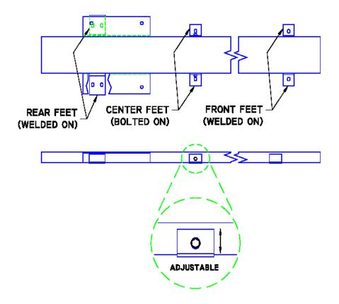
**Fig.2** Incorrect placement of the center adjustable feet can cause the bedplate to be drawn down in the middle when the mounting bolts are secured. **This will result in alignment problems with the pump, motor, and the suction plumbing of the RO unit.**
